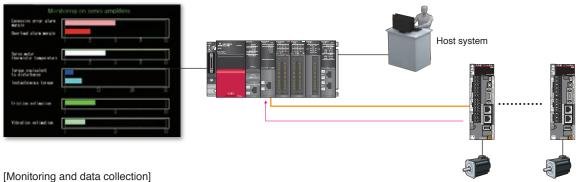
Alarm history of servo amplifiers (Note), Power consumption, 7-segment LED display status (Note), Identification information of servo amplifiers and servo motors (Note),
